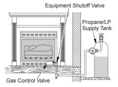
Figure 25 - Checking Gas Joints for Propane/LP Gas
